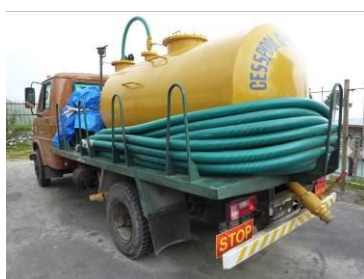
Figure 40: Cesspool truck recently acquired for desludging operations in Tsimasham/Tsimalakha
