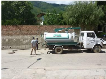
Figure 38: Discharge of collected sludge in a sewer manhole
